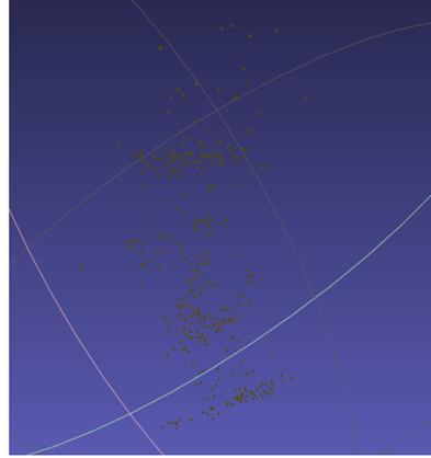
(b) Sparse Point Cloud Reconstruction using SURF
